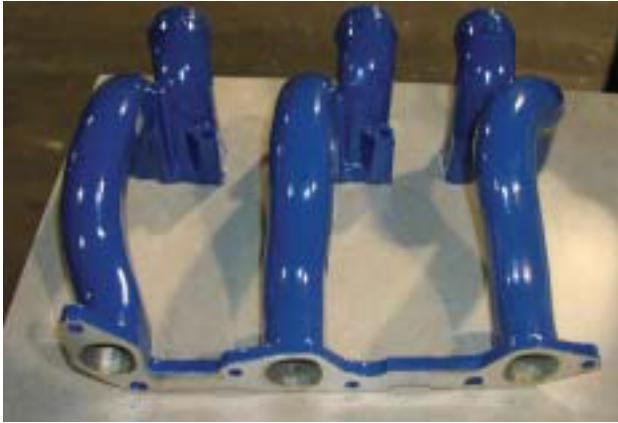
***The intake manifold was Plaforized and then powder coated blue.***
