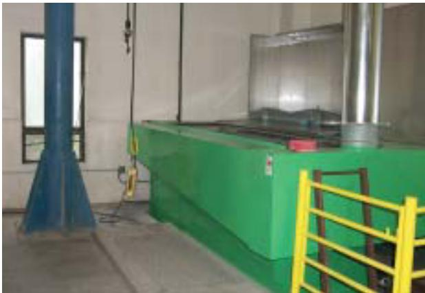
***This larger dip tank has an overhead hoist.***
