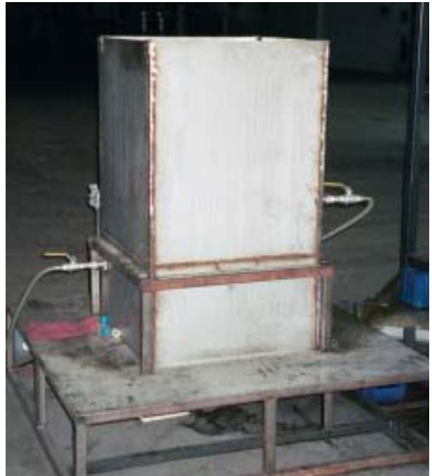
***A small dip tank is used for Plaforization of parts at Smart Manufacturing, Schoolcraft, Mich.***
