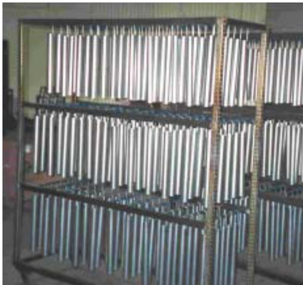
**Parts can be densely racked for treatment in the dip tank.**
