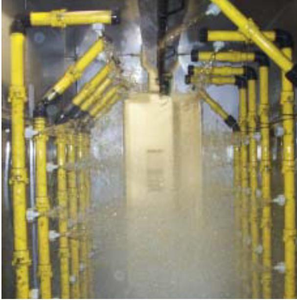
**Parts being treated in a spray operation.**
